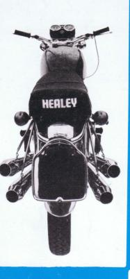
50 bhp at 6000 rpm, ten bhp more than the old Ariel "Square Four", and 80 lbs less in weight. It all adds up to performance.
