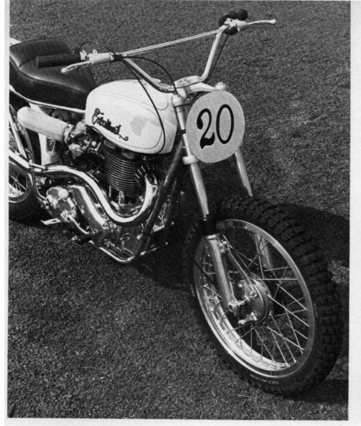
First the frame was completely nickel plated and all fittings were replated with cadmium. The gearbox was overhauled and the original wet clutch plates were replaced with dry ones.
