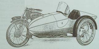
SUPER SPORTS SIDECAR MODEL V. Torpedo shaped body of large dimen sions. Spring seating cushion. Swing back cushion giving access to large compartment at rear. Blue leatherette upholstery. Body finished with weatherproof £22.10 labric (aluminium finish) and blue beading. Mat, coverall apron and wind screen
