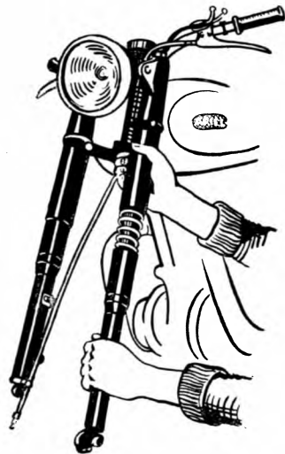
Fig. 22. Removing sliding tube and mainshaft after unscrewing "P" Plug.
